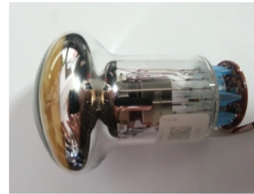
FIG. 87. A Hamamatsu R12199-02 7.7 cm PMT that is currently used in KM3NeT and considered for IceCube-Gen2 modules. As this passed the Hyper-K PMT requirements, it is also a good candidate for a Hyper-K mPMT.
