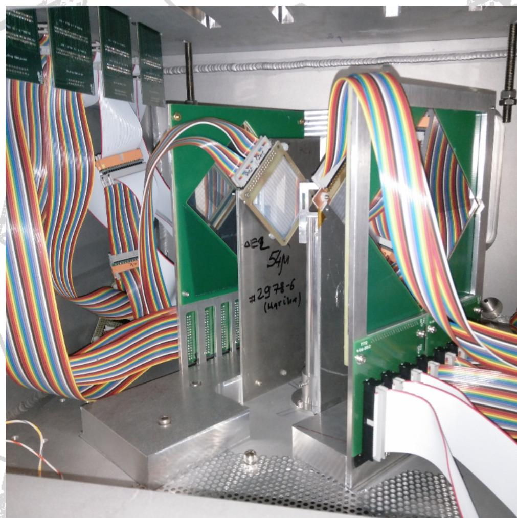
Detector Setup measuring  $^{10}\text{C}$  from reactions
