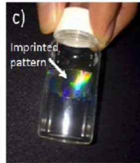
Grating on a curved glass vial surface
