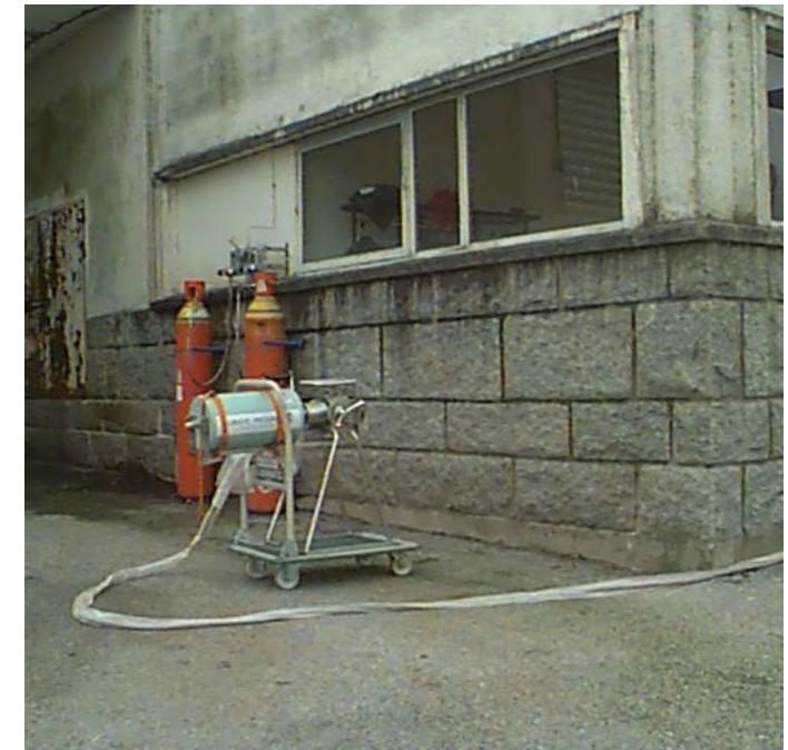
High efficiency HP Ge with tungsten shield
