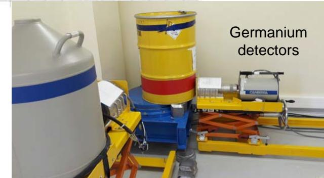
**Radionuclide activities:**  $A(E) = \frac{\varepsilon(E) \times I(E) \times T}{\text{Gamma-ray intensity}} \longrightarrow \text{Measurement time}$
