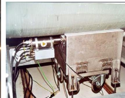
Measurement of the uranium enrichment in an UF<sub>6</sub> container by active neutron interrogation
