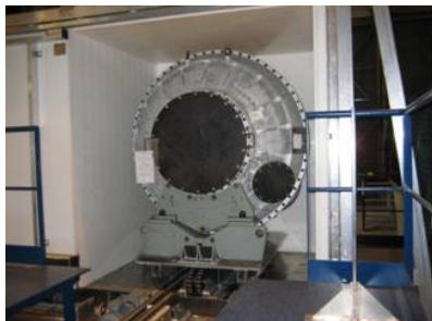
Passive neutron measurement of the uranium hold-up in UF<sub>6</sub> compressors
