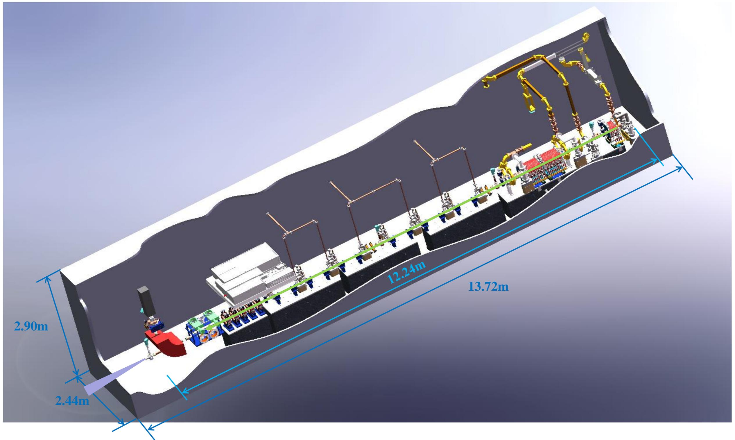
Main structures can be installed into a standard container.
