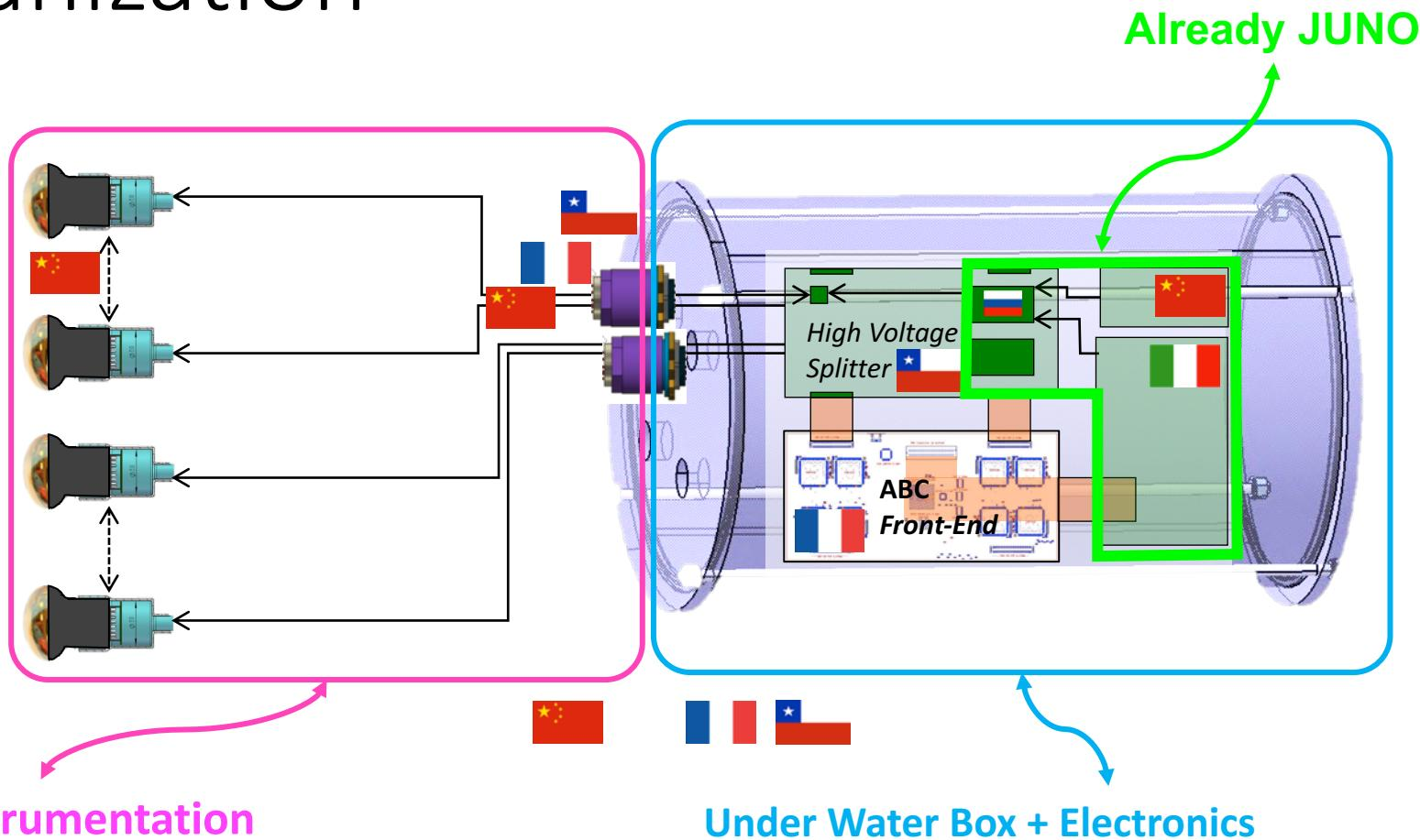
PMT instrumentation and UWB + Electronics are produced at different time, tested separately, and then installed together in JUNO → **underwater connector**
