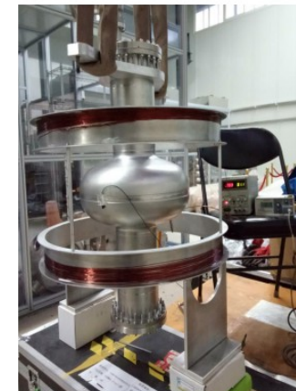
Helmholtz coil & flux gate for high Q research
