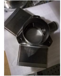
650 MHz 5-cell cavity with waveguide HOM coupler
