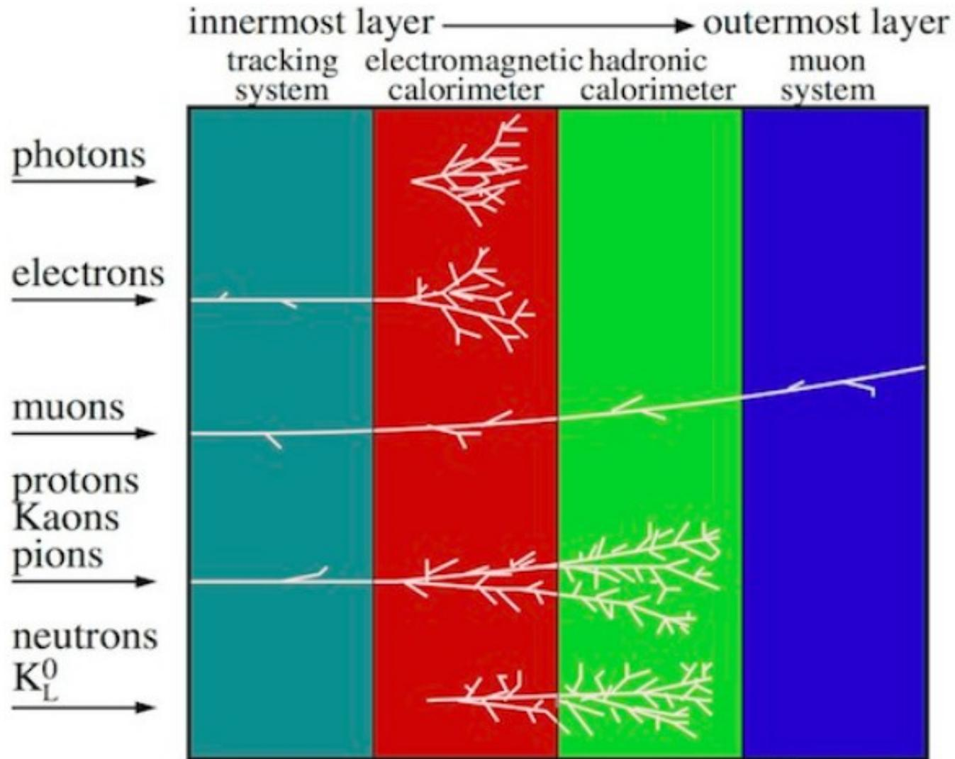
**Each particle type has its own signature in the detector.**
