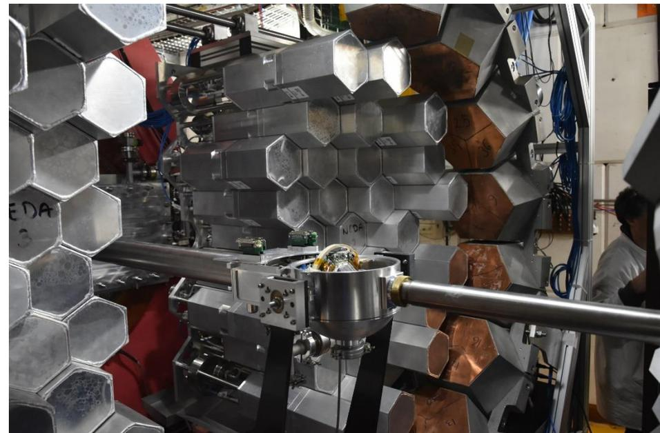
54 self produced NEDA detectors at forward angles and 14 NWALL detectors + plunger
