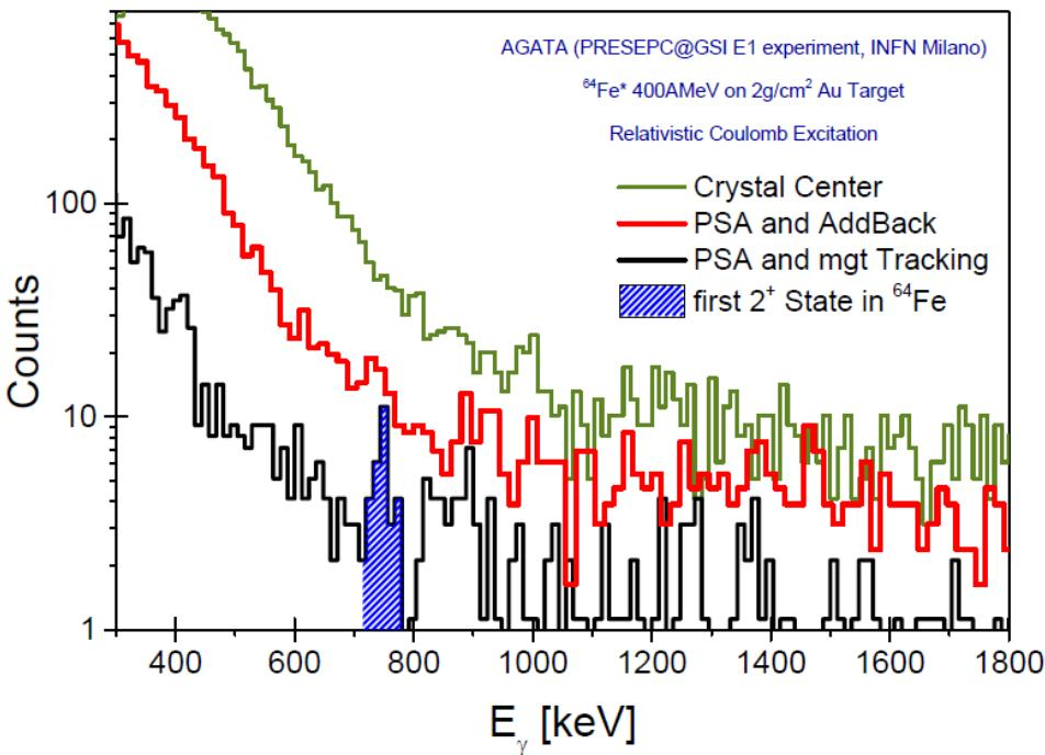
Measurement of known 2<sup>+</sup> states (needed to «calibrate» E1 strength) proofs that AGATA & Prespec PSA+Tracking setup works very well at E\_beam=440AMeV !!!!
