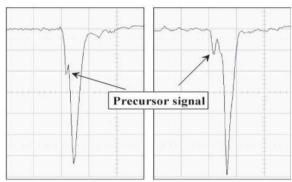
RPC signals (gas mixture with SF6) (from NIM A457 (2001) 117-125 )
