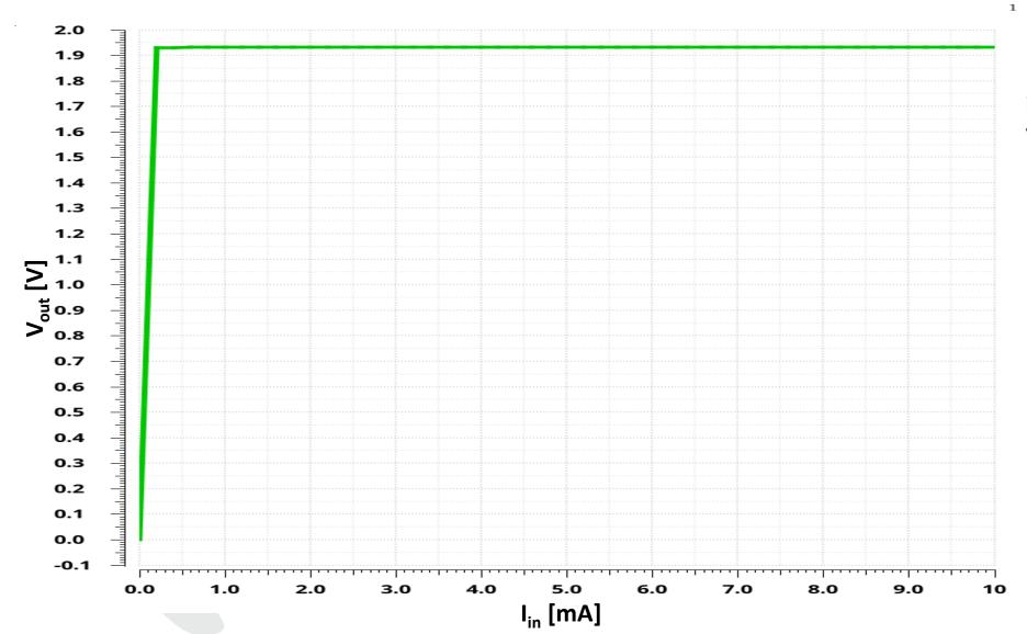
In DC, the regulator acts as an ideal voltage source in series with  $R_0 = 175 \text{ m}\Omega$
