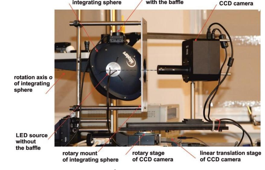
Laboratory setup to measure angular properties
