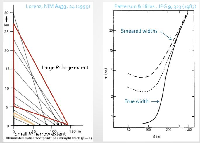
At sufficiently high energies, larger detector spacings can be used to measure the time-width at a given *R*.
