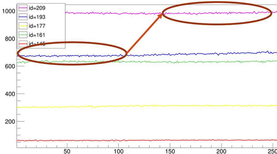
Slow mode of operation is useful for relative calibration and should be implemented in K-EUSO
