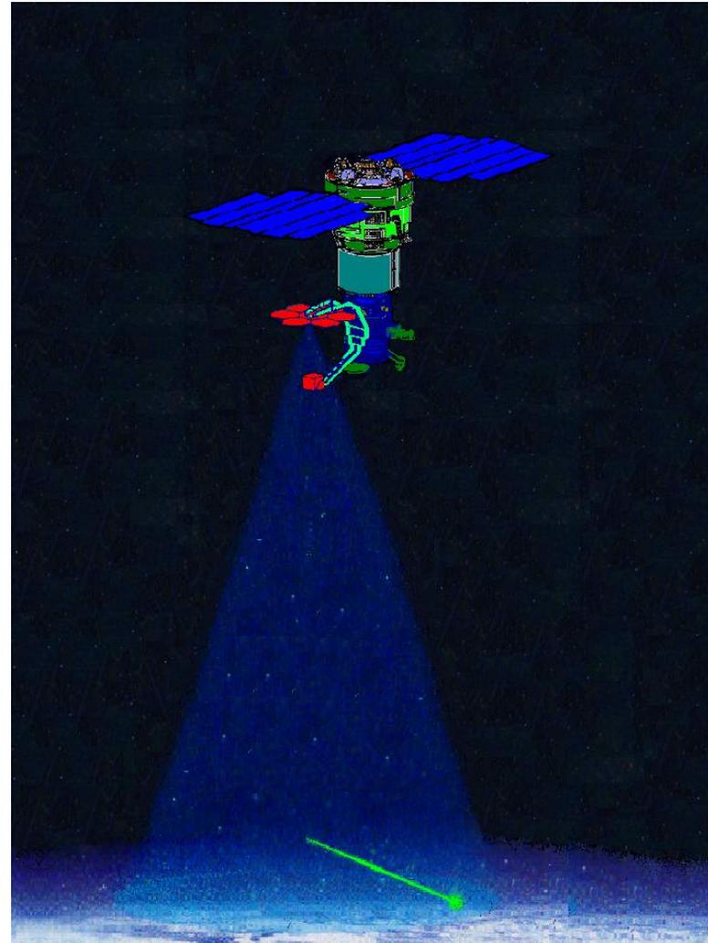
Detector TUS is designed as a multifunctional orbital telescope for various luminous atmospheric processes research.
