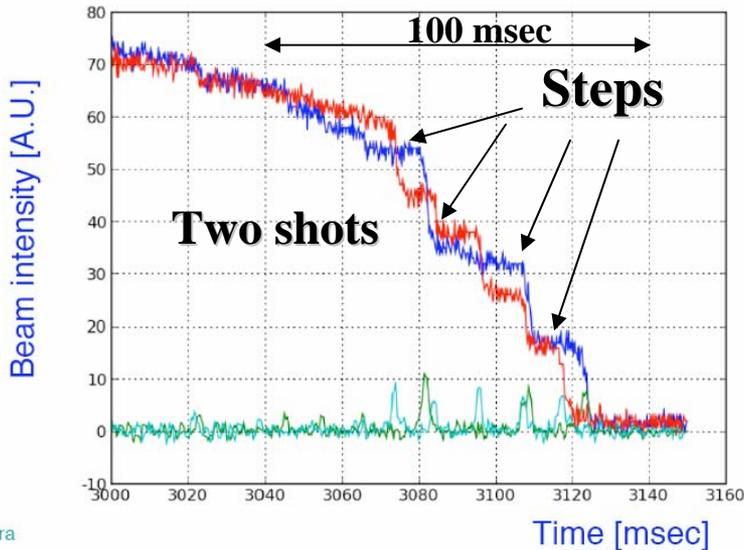
Spill measurement in HD beamline
