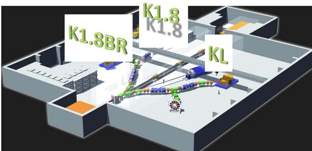
A possible layout of the beam lines at Hadron Facility.
