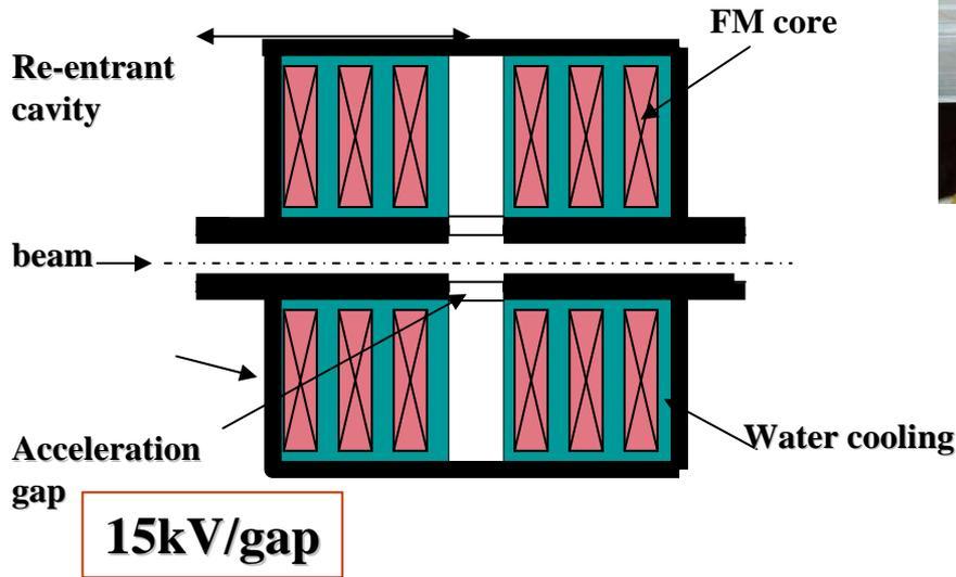
200 cores are used for RCS cavities
