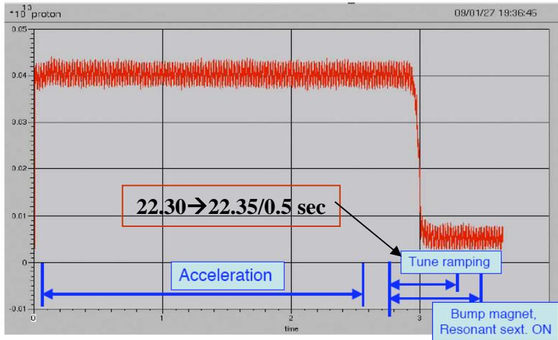
It's a "Ripple extraction" using SX system
