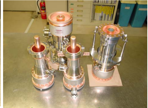
Cold couplers and warm couplers for STF phase-1 cryomodule
