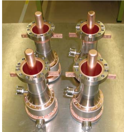
Cold couplers and warm couplers for STF phase-1 cryomodule
