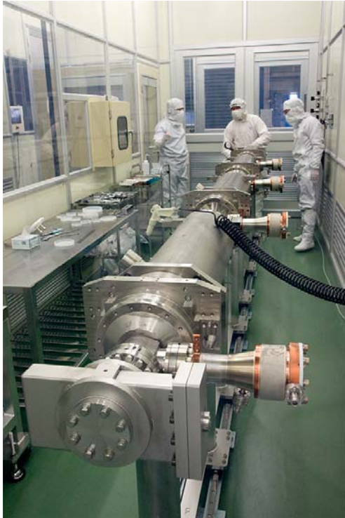
String assembly of four cavities & Installation of cold couplers
