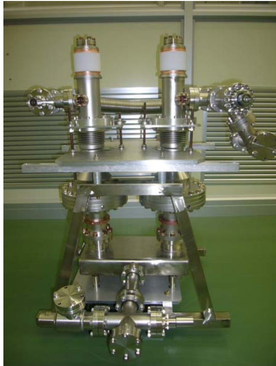
Assembly of pumping ports and vacuum gauges
