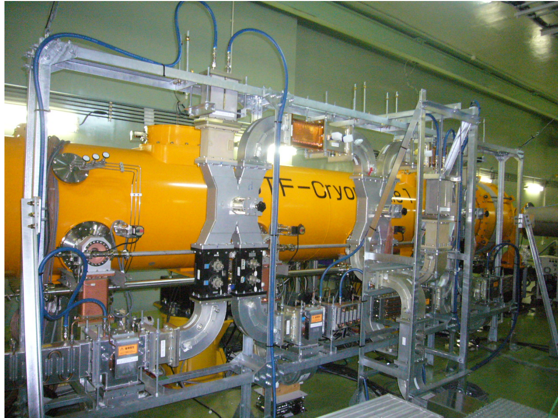
Installation of the cryomodule in the STF tunnel Connection with high power rf distribution system
