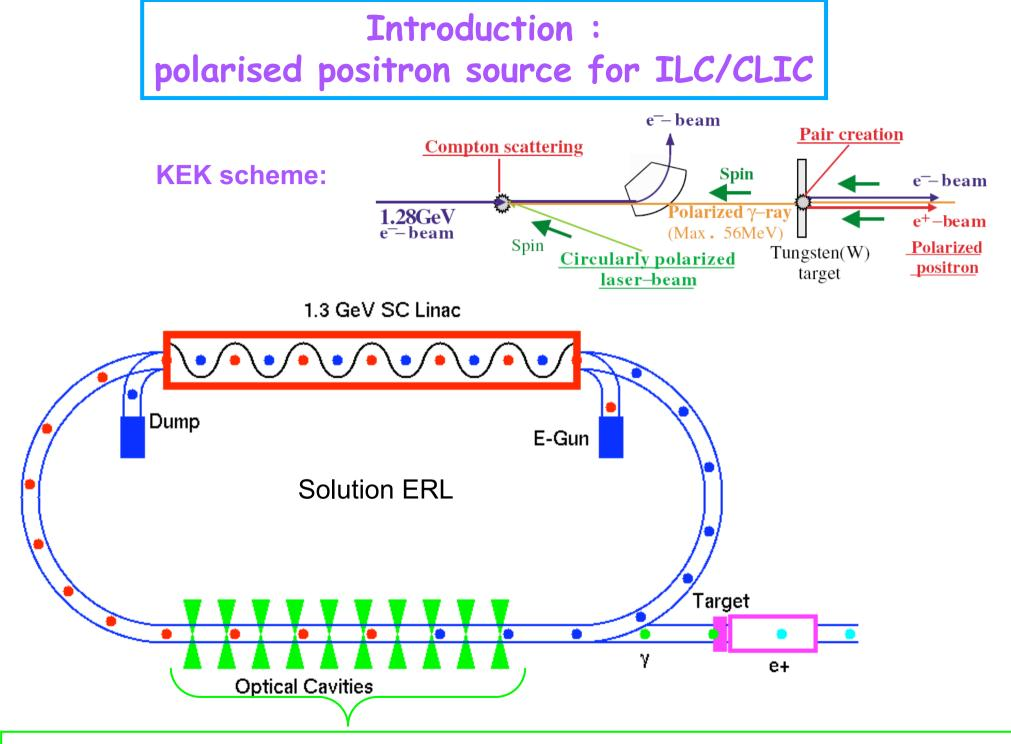
0.6J/pulse@1ps@60MHz  $\rightarrow$  <P>=36MW !!! per cavity  $\rightarrow$  R&D ! (KEK, LAL)
