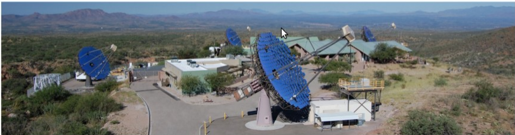
Figure 3.5.: Currently operating third generation IACT arrays: The MAGIC telescopes on La Palma, Canary Islands ( upper left , mirror diameters 17 m), the four H.E.S.S. telescopes (mirror diameters 12 m) and the large H.E.S.S. II telescope (average mirror diameter 28 m) on the Khomas Highland in Namibia ( upper right ), and the VERITAS array near Tucson, Arizona, USA ( bottom , mirror diameters 12 m). Image credits by the MAGIC/H.E.S.S. & VERITAS collaborations.
