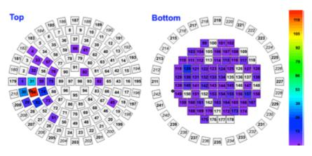
X and Y position from S2 hit pattern on the top PMTs
