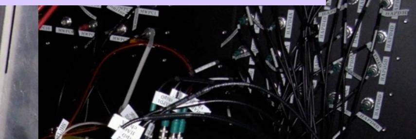
Front-end electronics attached at HAPDs
