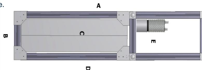
Fig 5: The prototype as used at the GSI test-beam in Aug '09. The bar on side A was Suprasil<sup>®</sup>-1 & the bar on side D was a totally absorbing dummy.
