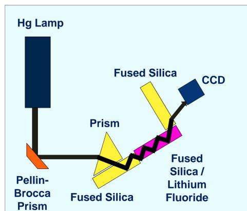
Fig 4: Initial set-up for testing chromatic dispersion correction properties of LiF
