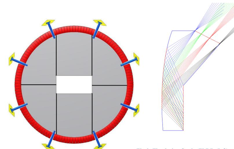
Fig 2: The design for the FLDD (left) and an example Focussing Lightguide (right)
