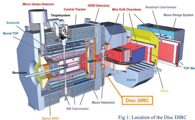
Fig 1: Location of the Disc DIRC within PANDA
