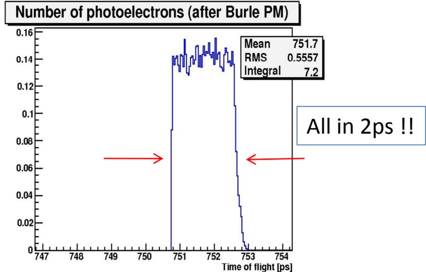
20cm  $\text{C}_4\text{F}_{10}$  + Flat mirror + central protons + 50% CE
