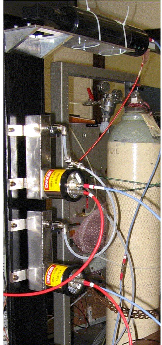
Dedicated picosecond laser test setup was developed to characterize fastest MCP-PMTs from Photek and Hamamatsu – using Agilent scope with 8 GHz BW and 40 GSamples/s
