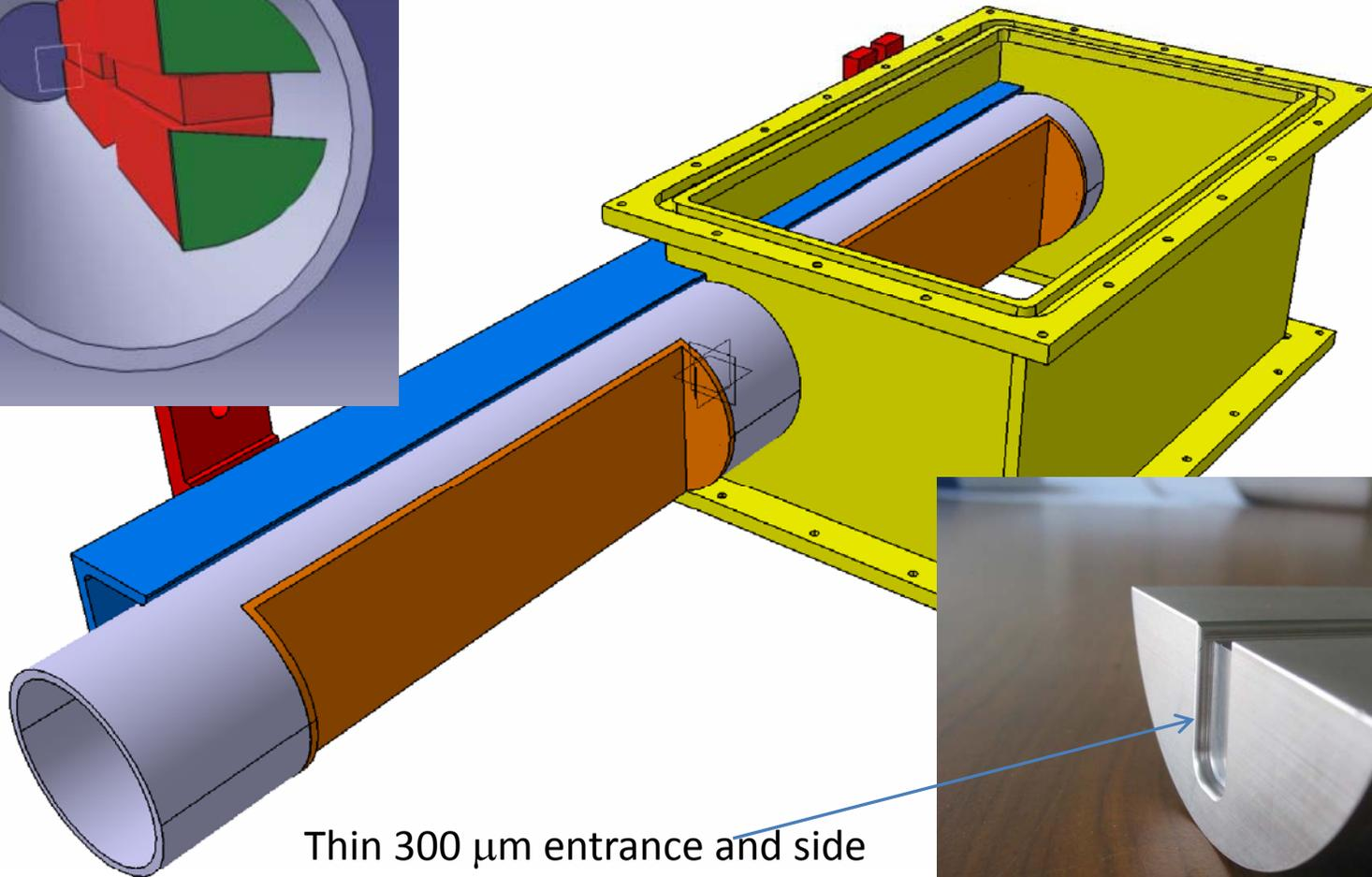
Thin 300  $\mu\text{m}$  entrance and side windows by electro-erosion
