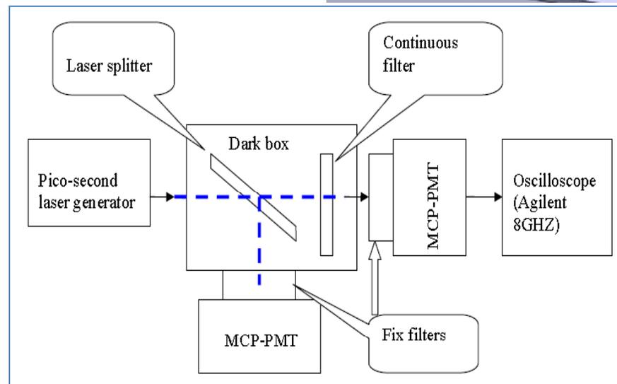
PiLas laser test setup runs up to 1 MHz repetition rate at 408 nm and using 8 GHz Agilent scope with 40 GSa/s
