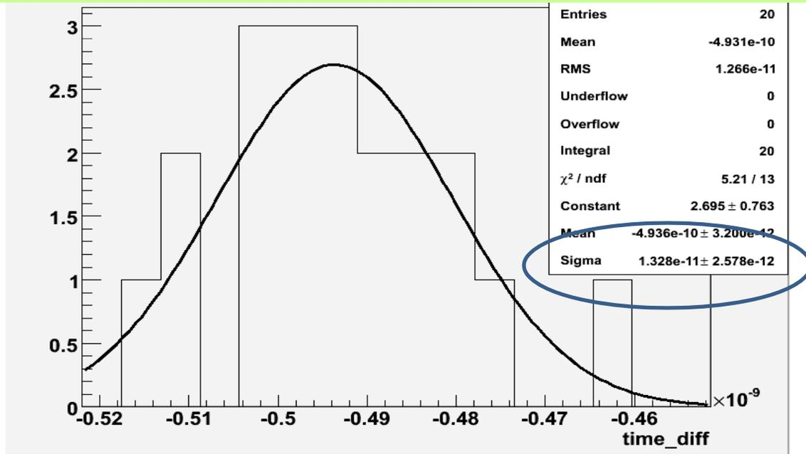
Example of time difference measurements of two GasToF detectors with Photek MCP-PMTs ;
