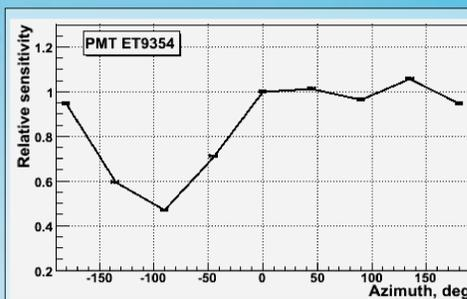
PMT's sensitivity depending on its azimuthal orientation. Photocathode's centre is illuminated.
