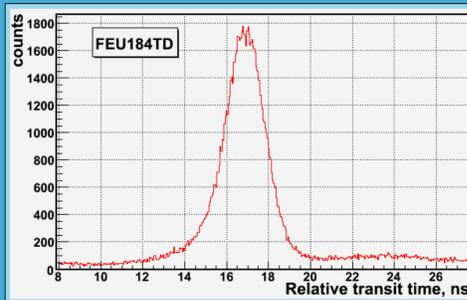
Single photoelectron jitter of PMT FEU184TD, main peak
