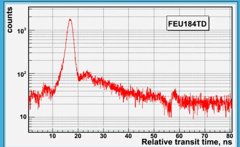
Single photoelectron jitter of PMT FEU184TD, main peak and tail
