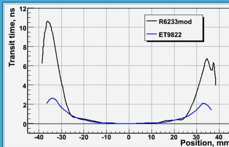
Transit times of fully (ET9822) and partly (R6233MOD) concave photocathodes
