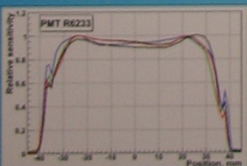
For most of the measured PMTs, the variation in relative sensitivity does not exceed 10%
