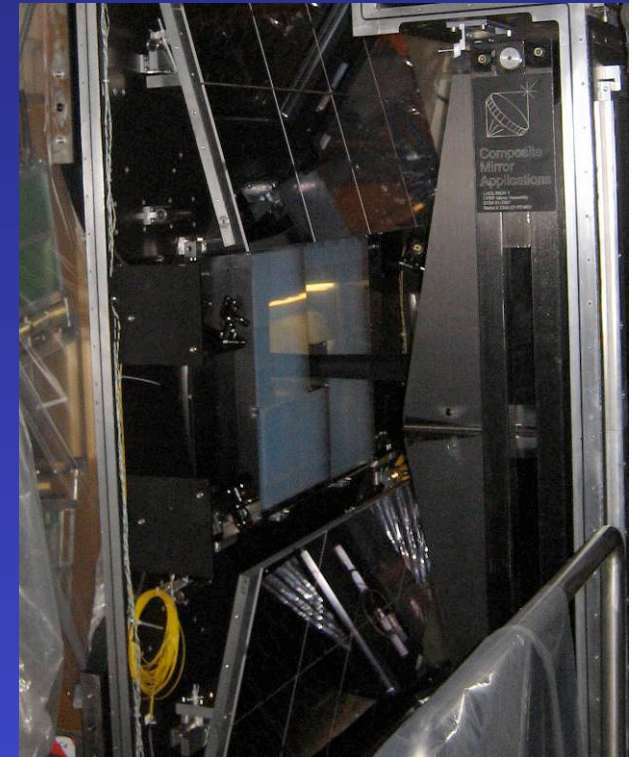
RICH 1 Inside gas enclosure with Aerogel and planar mirrors
