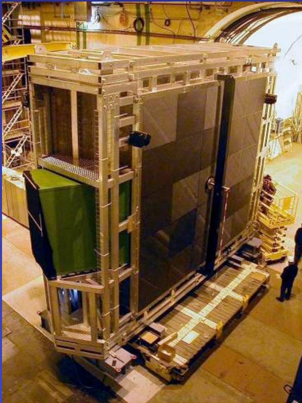
RICH 2 Detector Support structure, entrance window, magnetic shielding
