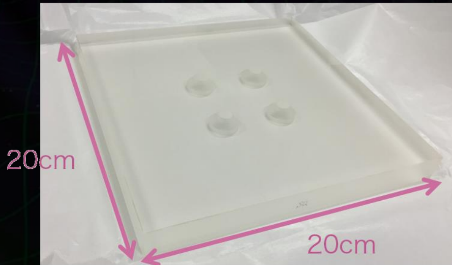
Fused Silica Optical Bench : \lambda polish for surfaces
