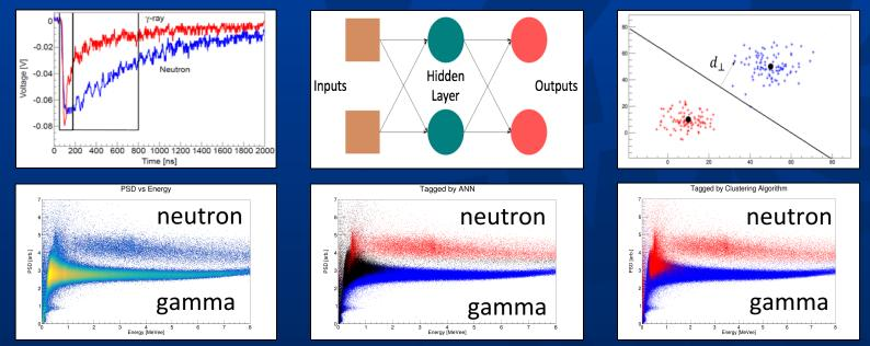
Machine learning algorithms capable of separating neutrons and gamma-rays in CLYC scintillators in the energy range investigated
