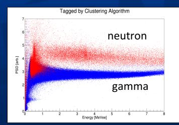
Machine learning algorithms capable of separating neutrons and gamma-rays in CLYC scintillators in the energy range investigated
