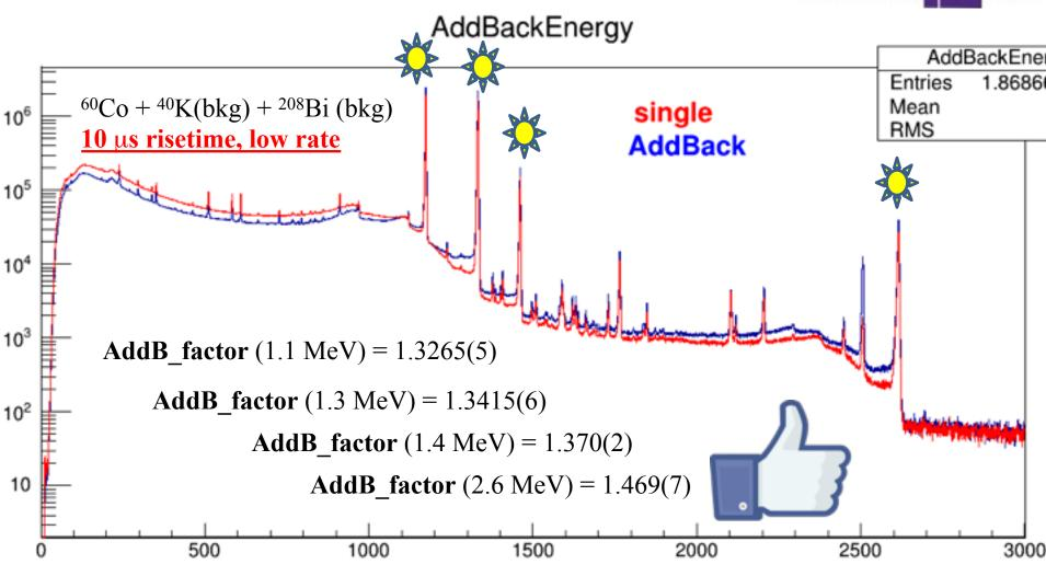
To make it easy: only core (E0) energies are considered. No Tracking but a simple AddBack procedure using neighboring cores **AddB\_factor** = Int(AddB)/Int(Single)
