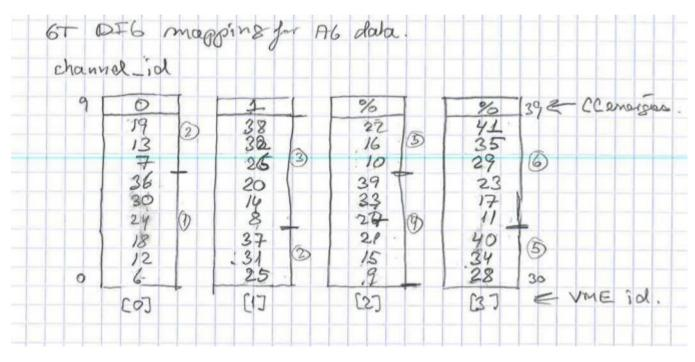
Mapping of AG segment channels into the four GT digitizers
