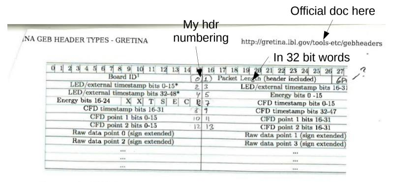
The energy is a 24-bit 2's complement signed integer, and must be converted to a 32-bit signed integer before use. The detector ID is a compound word consisting of 4 bit-fields as follows:
