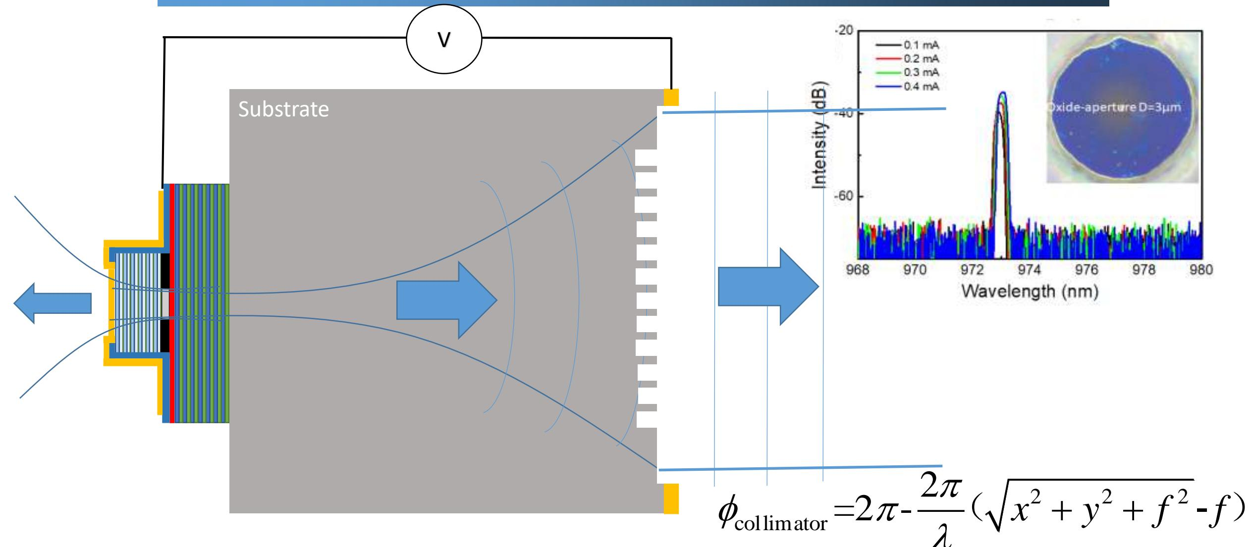
Electrically-pumped Vertical Cavity Metasurface-Emitting Lasers (VCSELs) for programmable directional lasing emissions
