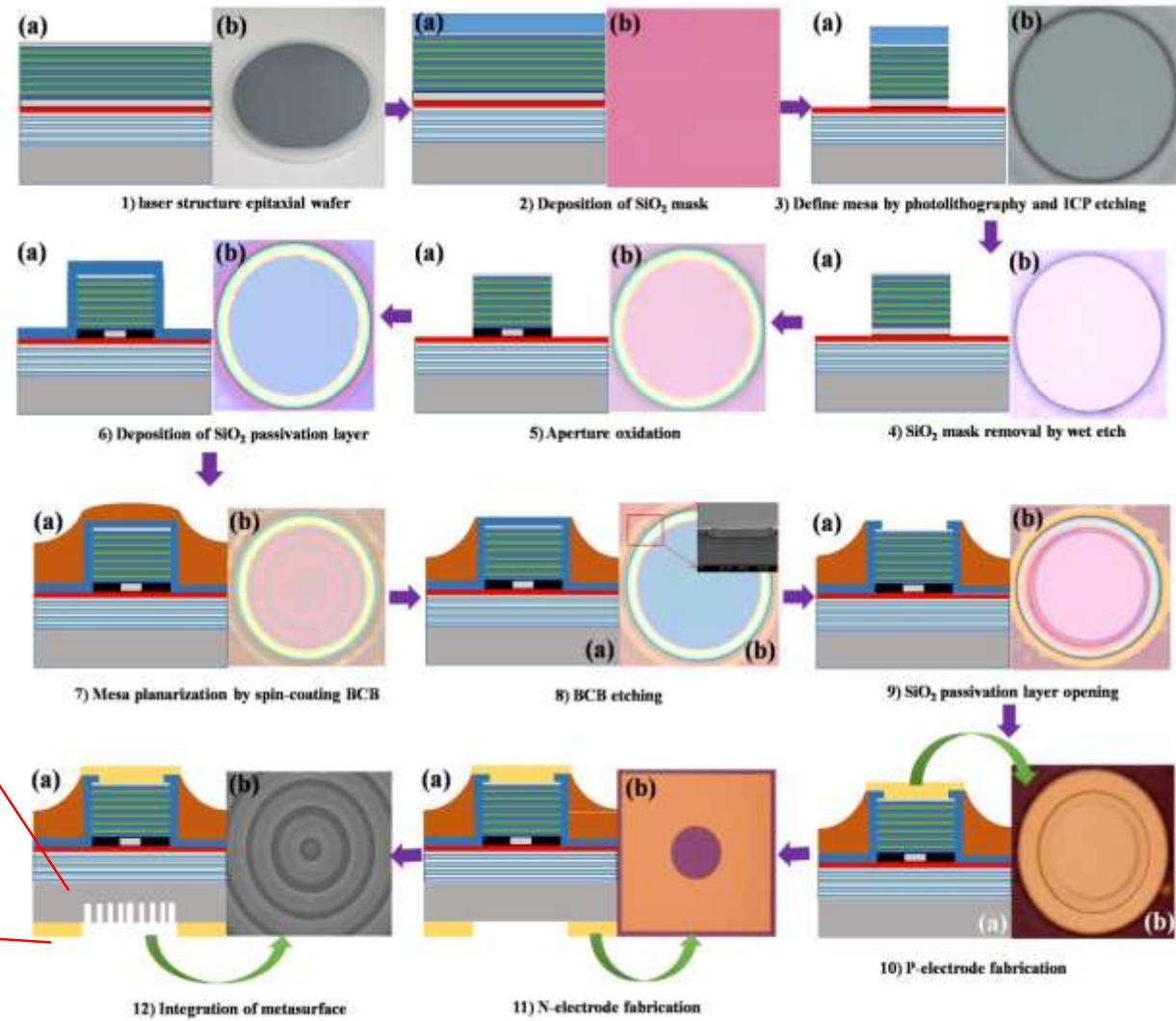
Electrically-pumped Vertical Cavity Metasurface-Emitting Lasers (VCMELs) for programmable directional lasing emissions
