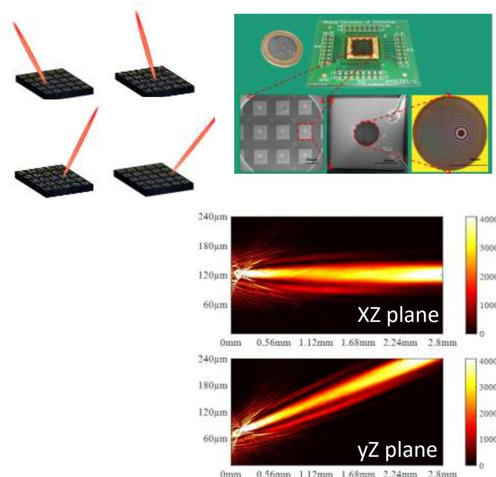
Electrically-pumped Vertical Cavity Metasurface-Emitting Lasers (VCMEs) for programmable directional lasing emissions
