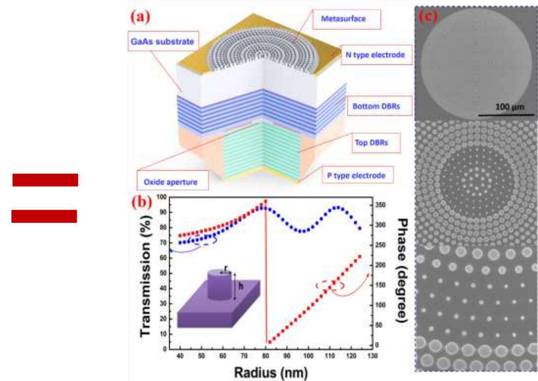
Self-collimated or nondiffracting Bessel laser
