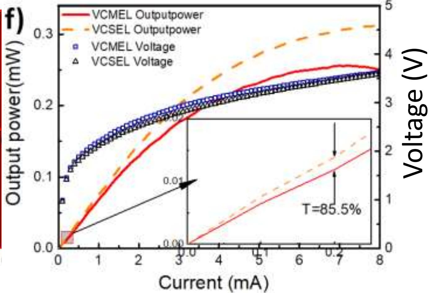
Electrically-pumped Vertical Cavity Metasurface-Emitting Lasers (VCSELs) for programmable directional lasing emissions
