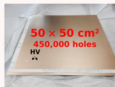
Fig. 7: A Large Electron Multiplier used in DLAr TPC (Fig 4)
