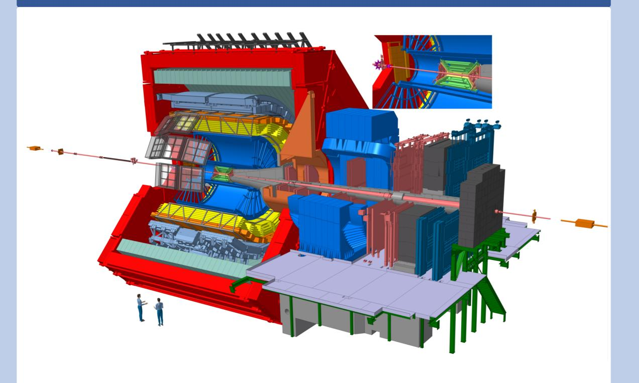
ALICE is a dedicated heavy ion experiment, composed of two main parts: the **Central Barrel** and the **Muon Spectrometer** in the forward region. The Muon Spectrometer covers the kinematic region  $-4 < \eta < -2.5$  and  $171^{\circ} < \theta < 178^{\circ}$ .
