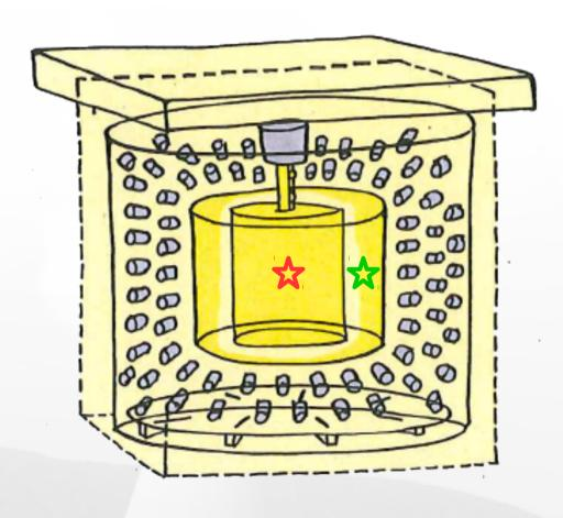
Use calibration source in **Target** and **Gamma Catcher** centers
