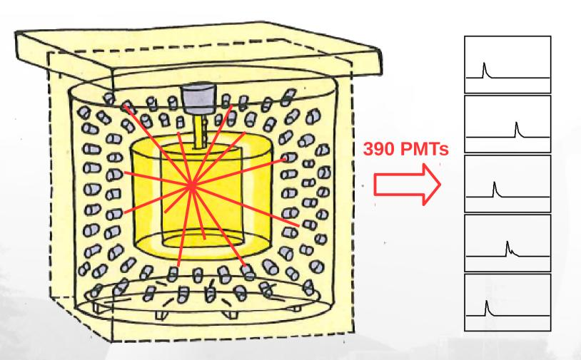
The scintillation waveform, as seen by the detector, is obtained by taking the 390 PMT signals, correcting them for the photon time of flight in the LS, and adding them up.
