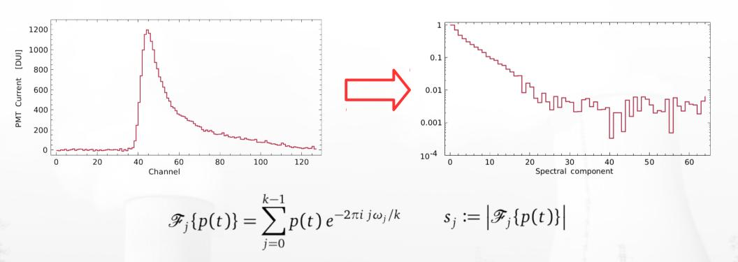
Power spectrum can reveal characteristics that are hidden in the time domain
