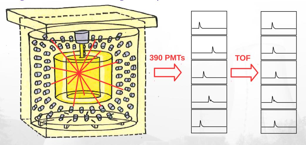
The scintillation waveform, as seen by the detector, is obtained by taking the 390 PMT signals, correcting them for the photon time of flight in the LS, and adding them up. The result looks more or less like this:
