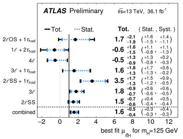
→ The combined signal strength is 1.6 <sup>+0.5</sup><sub>-0.4</sub>, which corresponds to 4.1σ (2.8σ) observed (expected) significance.
