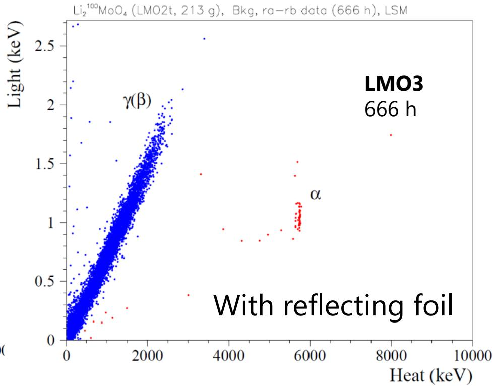
**Internal activity is compatible with  $b \sim 10^{-4} \text{ c/(keV kg y)}$**
