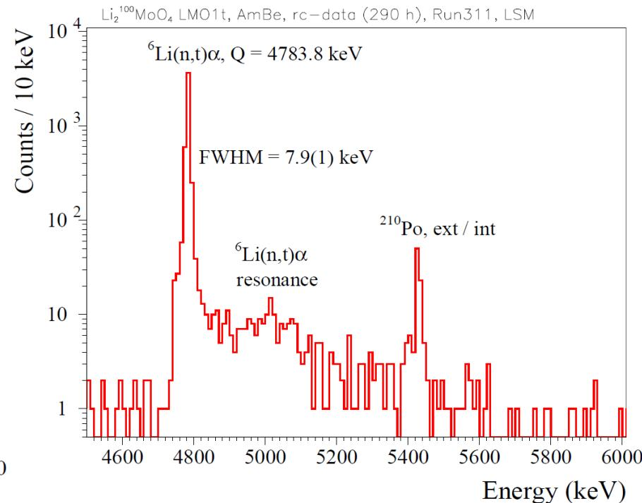
$\text{Li}_2^{100}\text{MoO}_4$  contains 7.6% of  ${}^6\text{Li}$  which allows to detect neutrons capture on Li: **world record resolution** of thermal n capture on  ${}^6\text{Li}$  (**FWHM = 6-11 keV at 4783 keV**)
