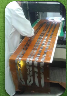
Long flex mixed Copper & stainless steel
