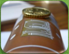
Embedded chip in low-mass aluminium flex
