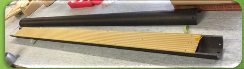
1.40m pcb coil to measure magnetic field
