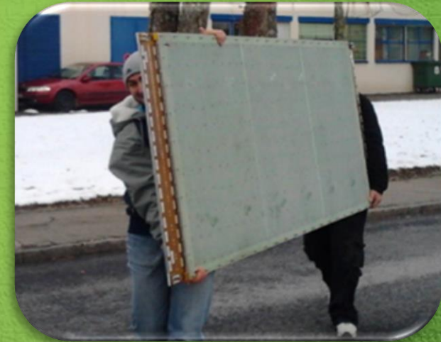
First Micromegas module 1 m x 2 m
