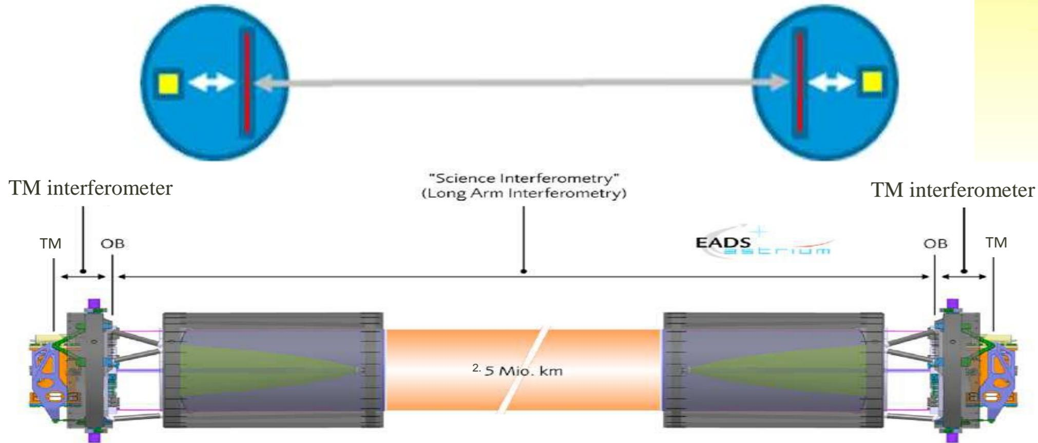
*Measurements to be performed are in the picometer range ( $1 \text{ pm} = 10^{-12} \text{ m}$ )*
