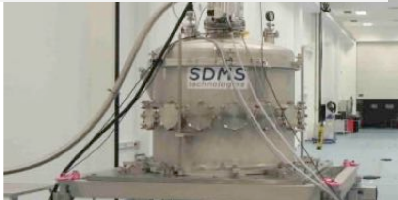
COL thermal vacuum chamber 0.2 m 3 – Top ~40K – P ~10 -6 mBar Designed for \mu -optical device testing
