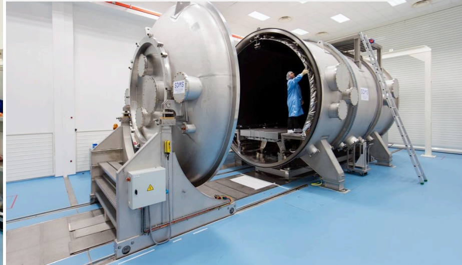
ERIOS thermal vacuum chamber 45 m 3 – currently ~80K – 10 -6 mBar Ultra-stable optical bench 10 -7 g
