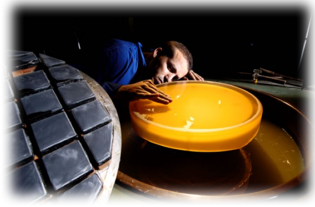
Polishing of the 40cm extreme quality active toric mirror for the VLT SPHERE
