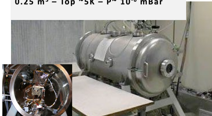
Herschel thermal vacuum chamber 0.25 m 3 – Top ~5K – P ~ 10 -6 mBar
