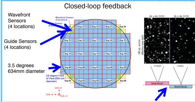
Simulated intra- and extra-focal images for one of the wavefront sensors, obtained using a simulation tool called PhoSim.
