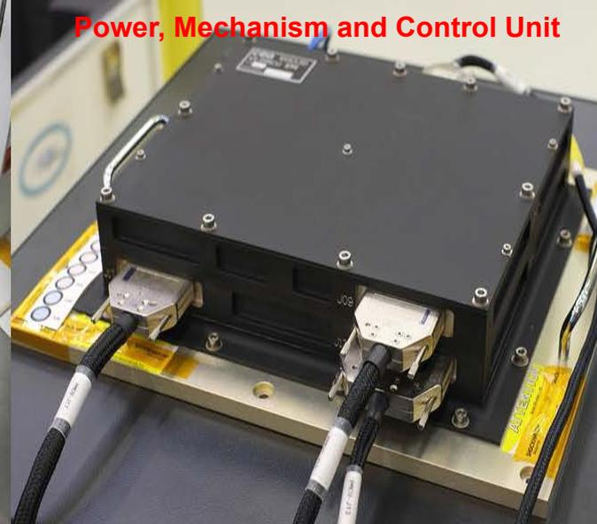
**Power, Mechanism and Control Unit**
