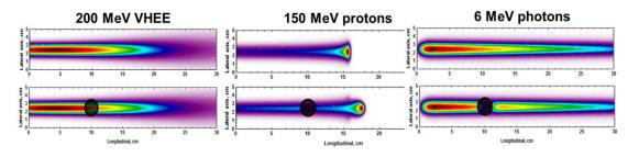
Behavior of VHEE, photon and proton beams traversing a air cavity (Agnese Lagzda, manchester)
