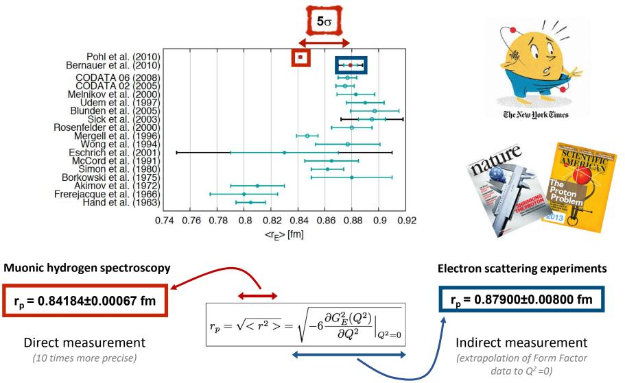
→ Problem: the proton is smaller as « seen » by muons than by electrons
