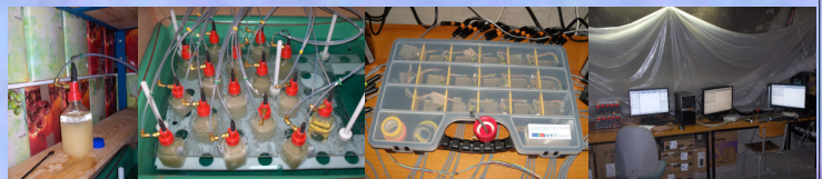
Fig. 6 Left to right: SDD with instrumented cap; SDDs in 9°C water pool; "Scorpions" box for the pre-amplification circuits and DAQ station at 1500 mwe
