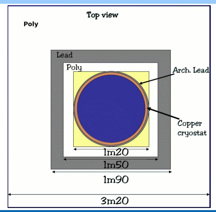
From external to internal the shield is made of:
