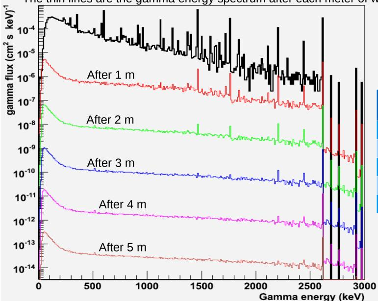
Total gamma flux outside the shield: 1.3 10<sup>-1</sup> (cm<sup>2</sup> s)<sup>-1</sup>
