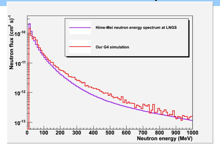
Another cross-check: we compared the shape of the neutron energy spectrum at the rock-hall boundary of our G4 simulation and the one obtained by Mei&Hime with Fluka.
