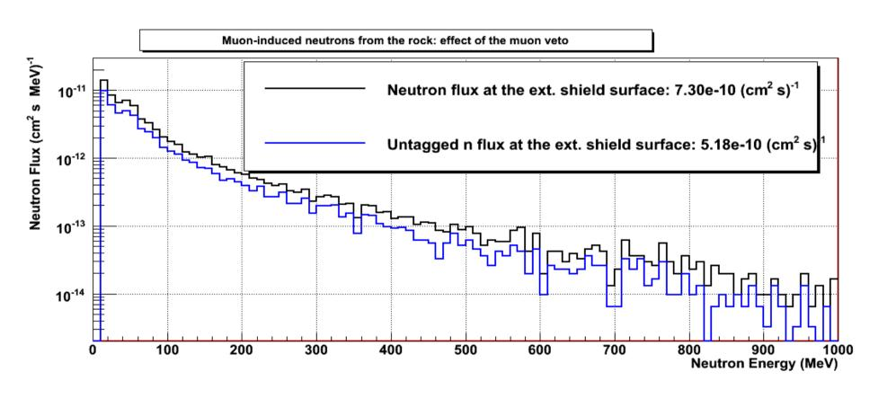
30% of the muon-induced neutrons are removed by tagging the corresponding muon with the water Cerenkov muon veto.
