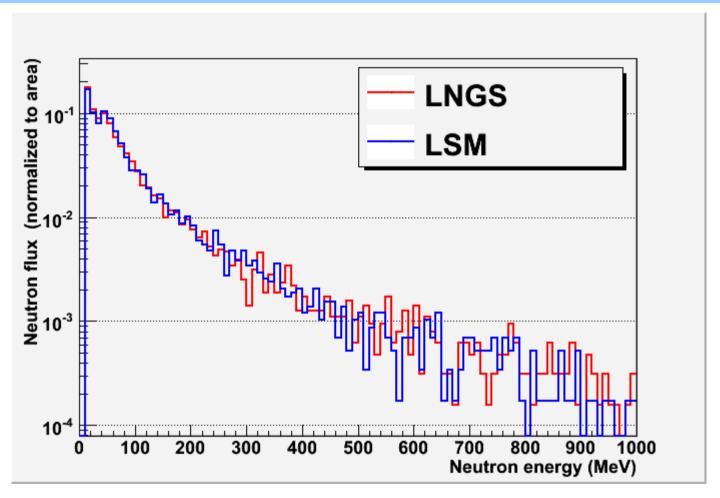
This is the neutron spectrum at the rock-hall surface, normalized to the same number of neutrons ... just to compare the shape of the two energy spectra. They are very similar for En>10 MeV.
