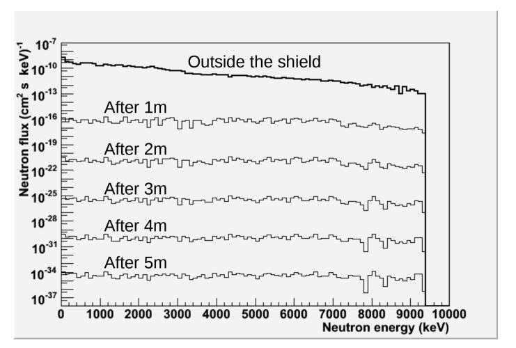
Total neutron flux outside the shield: 8.7 10<sup>-7</sup> n / (cm<sup>2</sup> s)
