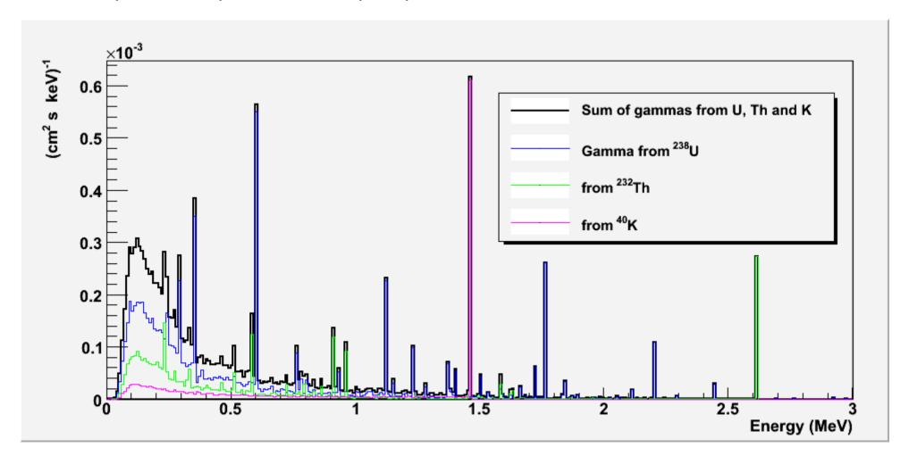
The total flux is 0.13 gamma / (cm<sup>2</sup> s) i.e. 1.13 10<sup>8</sup> gamma / (m<sup>2</sup> day)
