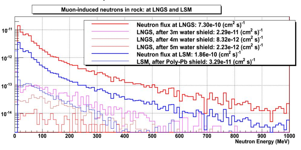
The <u>neutron flux</u> inside the <u>Poly-Pb shield</u> @ LSM is <u>of the same order of magnitude</u> of the one inside 3m of water @ LNGS.
