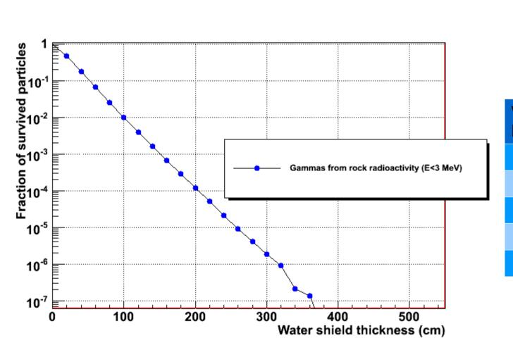
Total gamma flux outside the shield: 1.3 10<sup>-1</sup> (cm<sup>2</sup> s)<sup>-1</sup>
