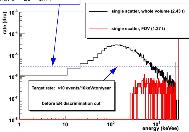
Conclusion: 3 m of water is well enough to shield external gammas.
