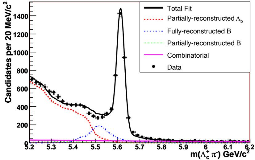
Figure 1: Unbinned maximum likelihood fit to the reconstructed invariant mass of  $\Lambda_b^0 \rightarrow \Lambda_c^+ \pi^-$  candidates. The fully reconstructed  $\Lambda_b^0$  modes (such as  $\Lambda_b^0 \rightarrow \Lambda_c^+ \pi^-$  and  $\Lambda_b^0 \rightarrow \Lambda_c^+ K^-$ ) are not shown separately on the figure.
