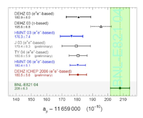
Whereas  $\tau$  based prediction agrees with the measurement within  $1\sigma$  all recent e+e- based predictions have a deviation with data at over  $3\sigma$
