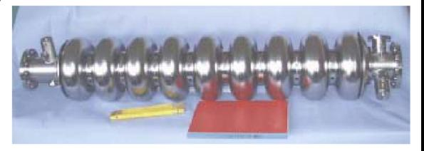
One standard 9-cell TESLA accelerating structure
