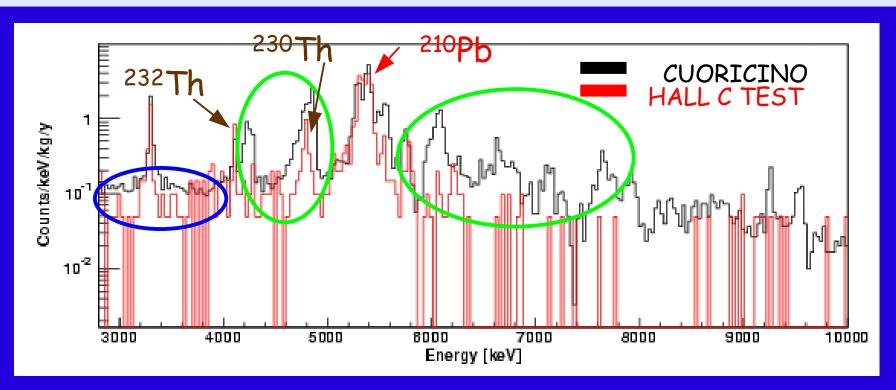
We were able to disentangle bulk vs. surface crystal contamination (Apparently crystals bulk has Th isotope contaminations, no evidence of U contamination in secular equilibrium)
