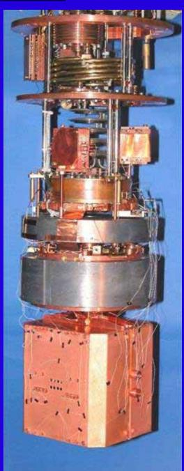
Cu: etching, electropolishing and passivation TeO2: etching and lapping with clean powders
