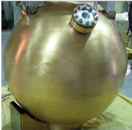
Left: Picture of SEDINE: a 60 cm diameter prototype made of low activity (NOSV) copper.
