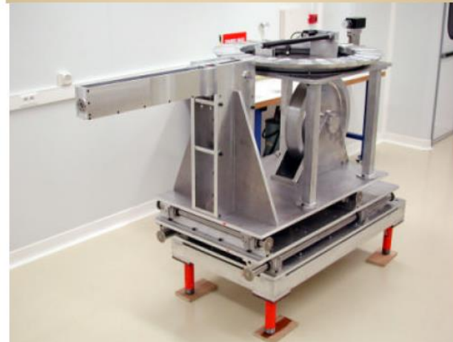
"Carousel" brick dispensing and storage system
