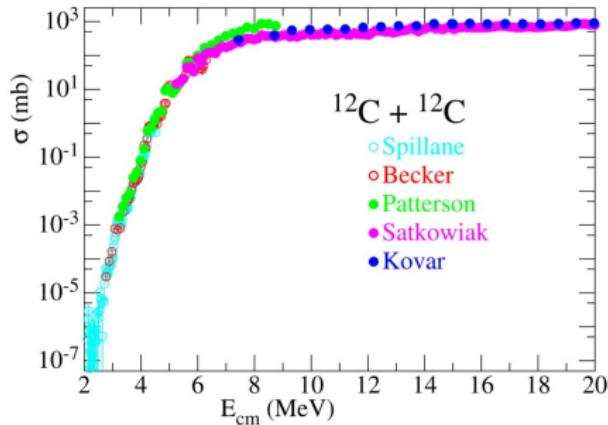
Previous fusion cross section measurements of  $^{12}\text{C} + ^{12}\text{C}$
