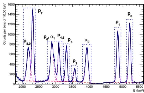
No coincident particle spectrum from S3B -  $E_{lab} = 11$  MeV
