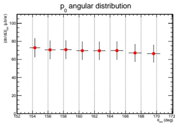
Angular distribution for the  $p_0$  exit channel -  $E_{lab} = 11$  MeV
