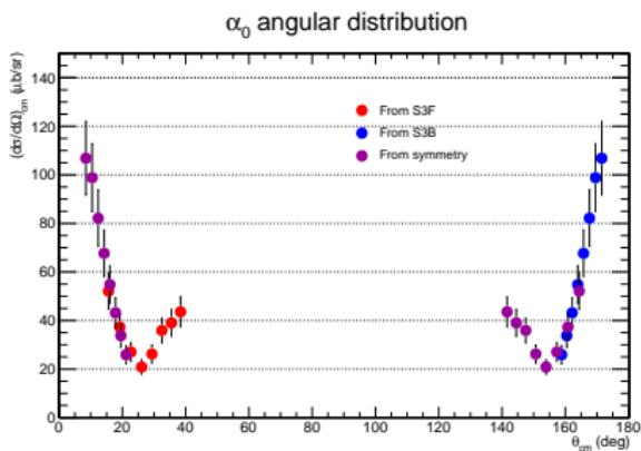
Angular distribution for the  $\alpha_0$  exit channel -  $E_{lab} = 10.8$  MeV
